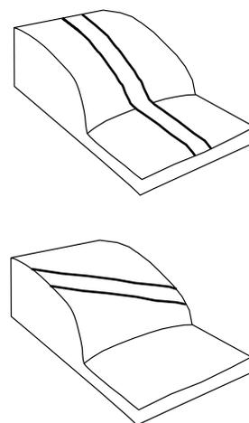
**Figure 6: Parallel-Slope (above) and Cross-Slope (below) roads.**
