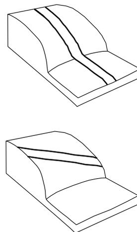
**Figure 6: Parallel-Slope (above) and Cross-Slope (below) roads.**
